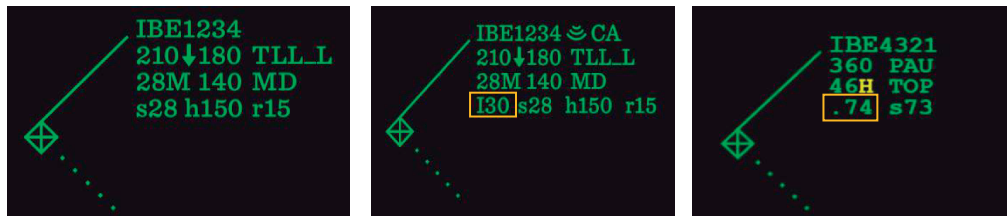
Figure 1: Current (left), proposed (middle) flight label and flight label showing MACH on CWP (right)
